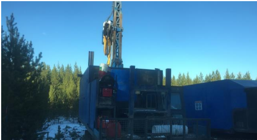
Reverse Circulation drill rig collecting Nechako till samples; bedrock was also sampled
